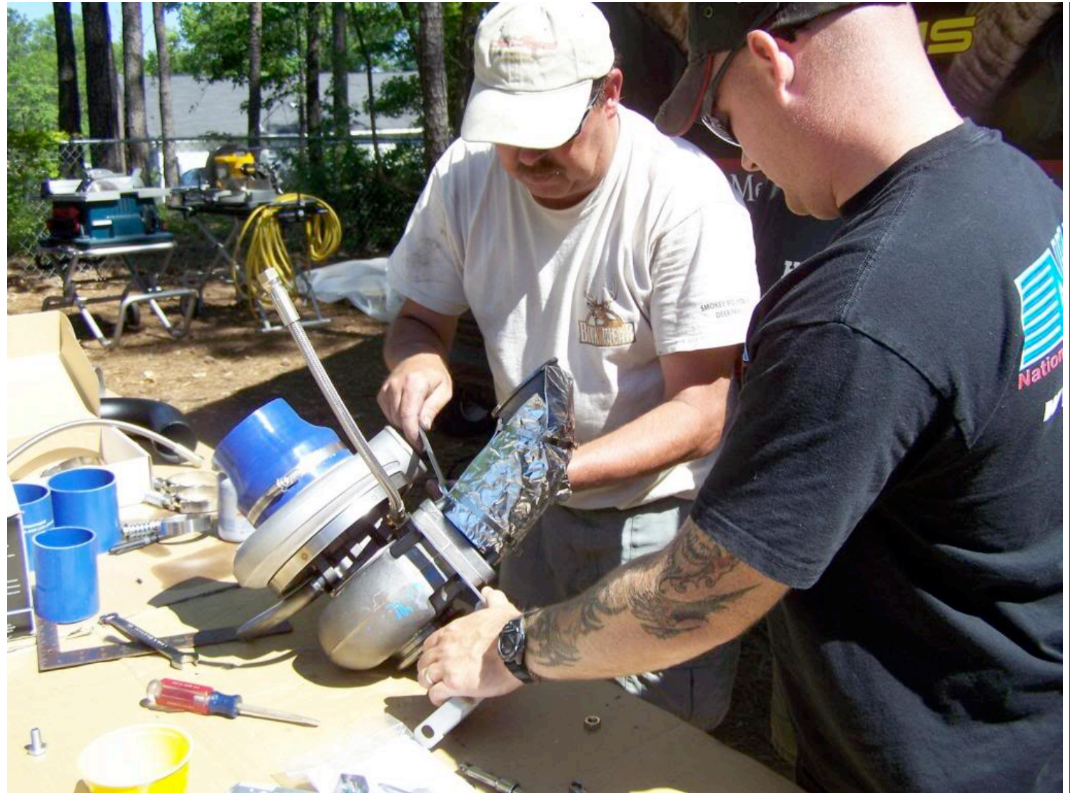
Once the primaries were positioned, we found the clocking that was called for in the BD directions was incorrect, so this was adjusted.
