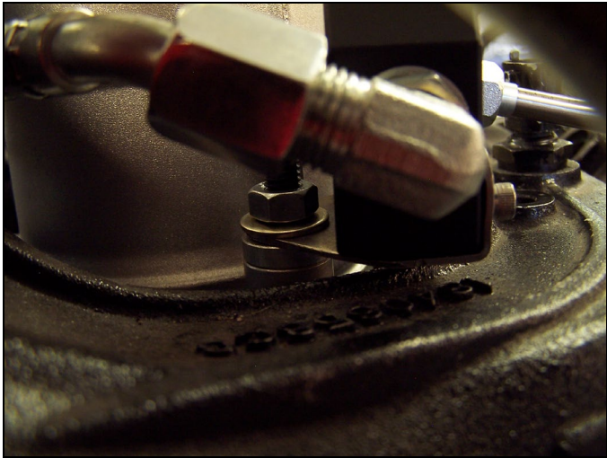
Spacers, Bracket, Top Washer and Nut Installed
