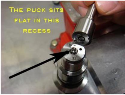
\*Note: For 5.9 injectors, there are two different style pucks that were in these units. Our nozzles will work with both designs shown here, simply follow the same install procedures.
