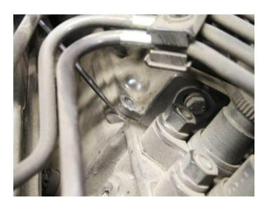
9. Remove the 2 8mm bolts holding the AFC, and the fuel shutoff solenoid.
