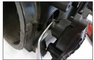
8. Pull the diverter door motor partially out of the air filter housing, then using a panel popper tool or similar device pry the diverter door off the motor shaft.
