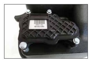
9. Install the diverter door motor onto the K&N air filter housing using the provided hardware.
