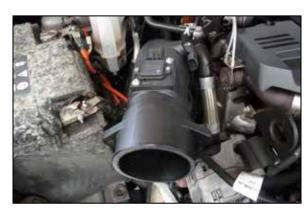
12. Install the K&N intake tube into the factory turbo inlet elbow, do not tighten the hose clamp.
