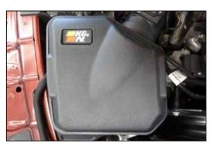
17. Install the K&N lid onto the air filter housing and snap the logo into the lid.
