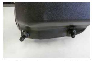
10. Install the mounting studs onto the K&N air filter housing using the provided hardware.
