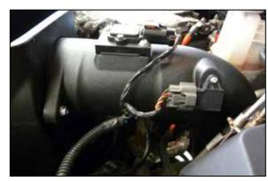
14. Reconnect the air sensor electrical connections.
