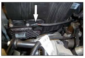
5. Lift the lower air filter housing up enough to gain access to the diverter door electrical connection, disconnect the diverter door electrical connection and then remove the lower air filter housing.
