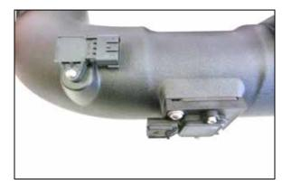
11. Install the two sensors into the K&N intake tube using the provided adapter and hardware.
