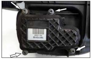
7. Remove the four bolts that secure the diverter door motor to the lower air filter housing.
