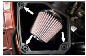
16. Install the three lid mounting grommets into the air filter housing.
