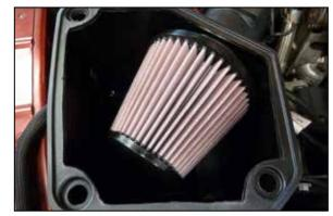
15. Install the K&N air filter onto the intake tube and secure with the provided hose clamp.
