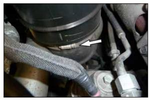
6. Loosen the hose clamp that secure the factory intake tube silencer to the turbo inlet elbow.
