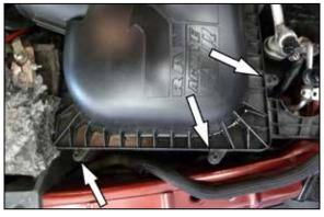
3. Loosen the three bolts that secure the air filter housing lid and then remove the lid.
