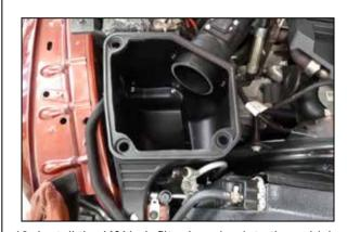
13. Install the K&N air filter housing into the vehicle so the mounting studs insert into the mounting grommets and the intake tube fits through the hole. Mount the tube to the air filter housing and the housing to the core support using the provided hardware. Tighten the hose clamp that secure the intake tube to the elbow.
