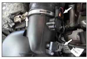
2. Loosen the hose clamp that secures the factory intake tube to the air filter housing. Disconnect the air sensor electrical connections.
