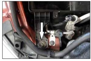
4. Remove the bolt that secures the lower air filter housing to the core support.
