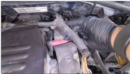
94. Connect Rear PCV Hose Back To Valve Cover
