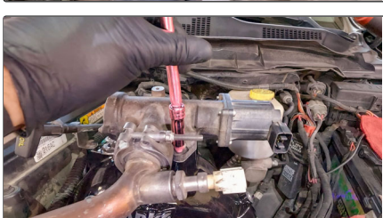
121A. Loosen Front Bolts on EGR Valve
