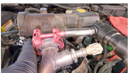
119A. Tighten Driver Side Clamp
