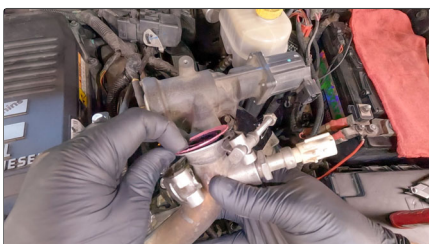
118A. Conical Gasket Goes On Driver Side of EGR Tube
