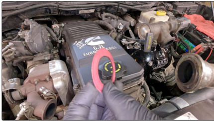
116A. Flat Washer Goes On Passenger Side of EGR Tube
