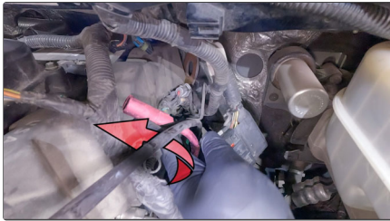
93. Run Rear PCV Hose Under Dipstick Tube
