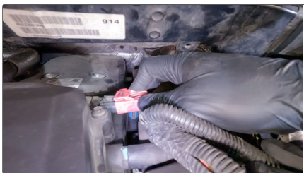
96. Connect Rear White Plug Be sure to slide the pink lock back into position.
