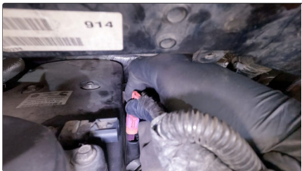
95. Connect Rear Flat Blue Injector Plug
