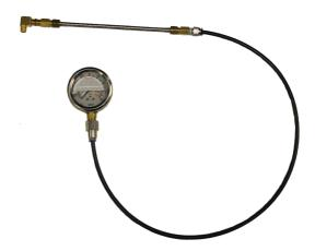
To test the idle pressures, the exhaust brake must be applied at idle. If the engine is cold, the brake will turn on when at idle, otherwise it must be commanded manually.
