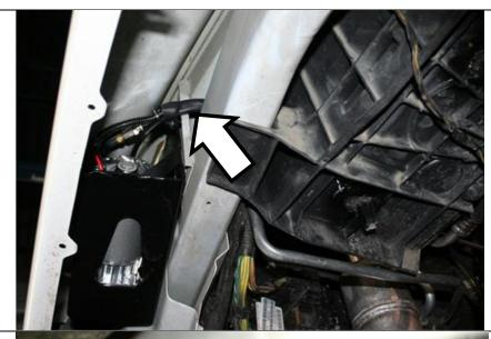
Secure the compressor in place by reinstalling the hood hinge bolt through the compressor bracket. Then install the nut and bolt to hold the front of the bracket.
