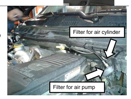
On 2007-2010 trucks, the preferred method of mounting the compressor air filter is just below the hood using a factory mounting location.
