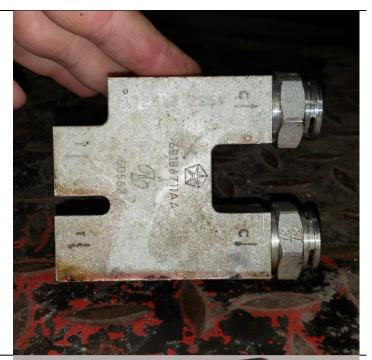
Install quick connect fittings (1300579) into BD Bypass block (1300580) using 1" and 24mm open wrench.
