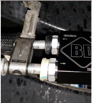
Inspect original O-ring on the tube, replace with supplied Viton O-ring (1453153) if damaged.
