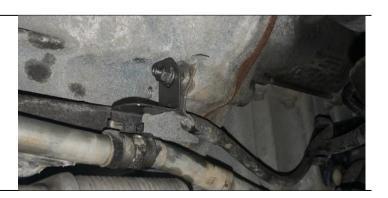
Reconnect the cooler tube retainer.
