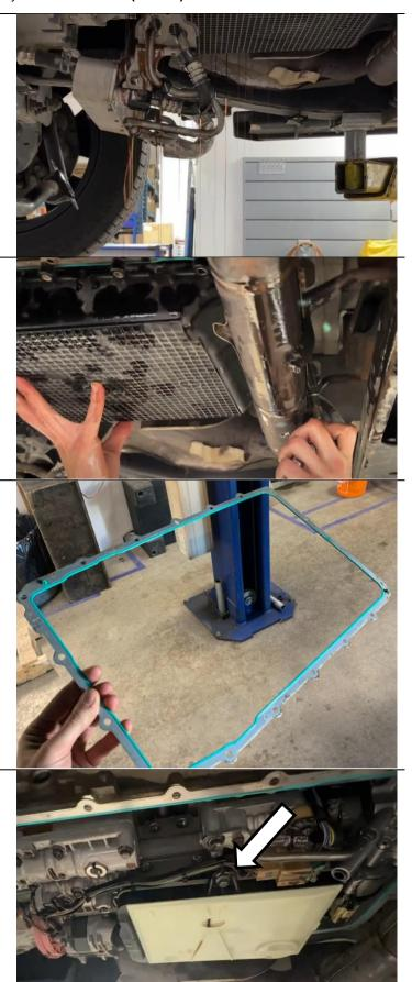
Wipe down the inside of the new pan with brake parts cleaner or another suitable substitute.
