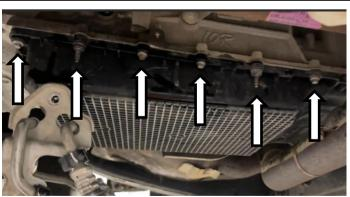
Slowly loosen and remove the bolts from front to back to allow the fluid to slowly drain out of the front of the pan.
