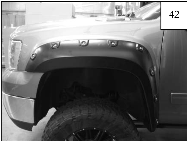
Reinstall wheel. Completed front flare installation.
