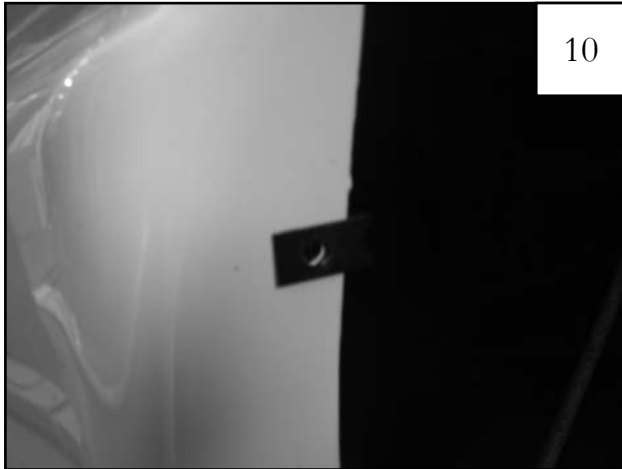
Install Clip (CL1-0011) over existing factory hole.
