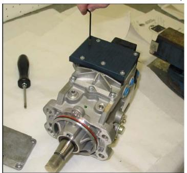
Place the piercing Allen set screw (*P/N#* 1502005) into the small hole on the plastic cover, and then screw it down with the supplied Allen key (*P/N#* 1502003) so that it is going in straight.
