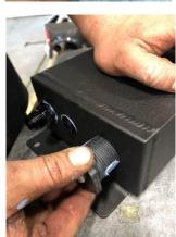
STEP 3: With all fittings installed into the tank, install the tank onto the battery box using the mounting hardware. The coolant tank will use existing holes in the battery box for mounting.
