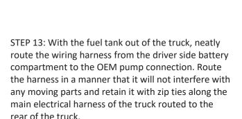
NOTE: The Fleece supplied wiring harness is required to power the secondary pump and handle the additional current draw.
