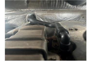
**STEP 3:** Disconnect the upper heater core hose from the quick disconnect fitting on the passenger side of the cylinder head. Use a flat head screwdriver to pry the hose adapter off of the fitting. Remove the upper heater core hose from the engine bay.
