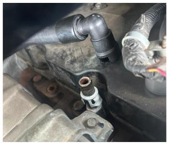
**STEP 5:** Apply thread sealant in a single bead around the lowest thread of the new heater core quick disconnect fitting.
