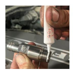
**STEP 6:** Using a 7/8" deep well socket or wrench, install the quick disconnect fitting into the cylinder head where the OE fitting was removed.
