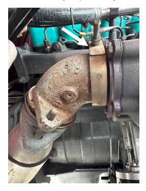
4. Disconnect the turbocharger oil supply line and the oil drain tube from the turbocharger. Discard the original turbocharger oil drain tube gasket.
