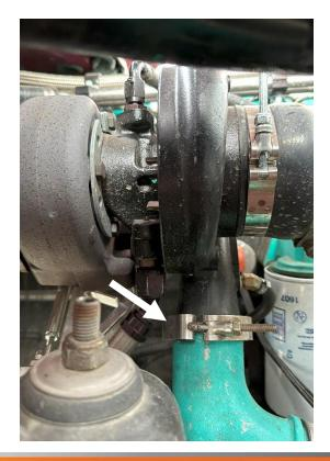
6. Remove the four turbocharger mounting nuts from the manifold and turbocharger. Remove the turbine flange gasket from the exhaust manifold. Discard the original manifold gasket, nuts, and studs.
