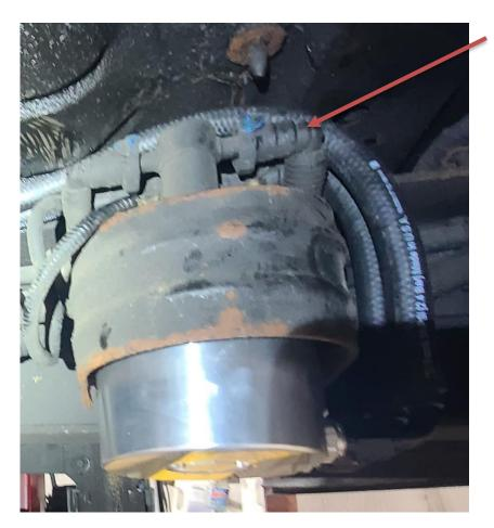
5. The factory return line will get connected to the horizontal fitting on the return filter head that points towards the front of the truck. When connecting the fuel lines, ensure that they are fully locked onto the quick connect fittings.
