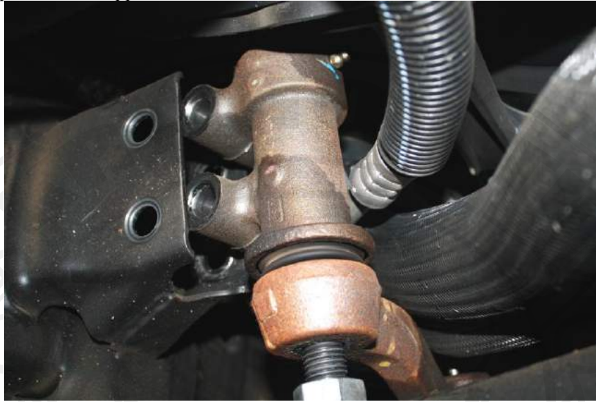
Figure 8: idler arm and idler pivot
