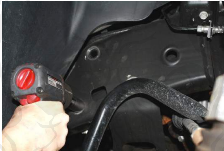
Figure 6: unbolt steering box from frame
