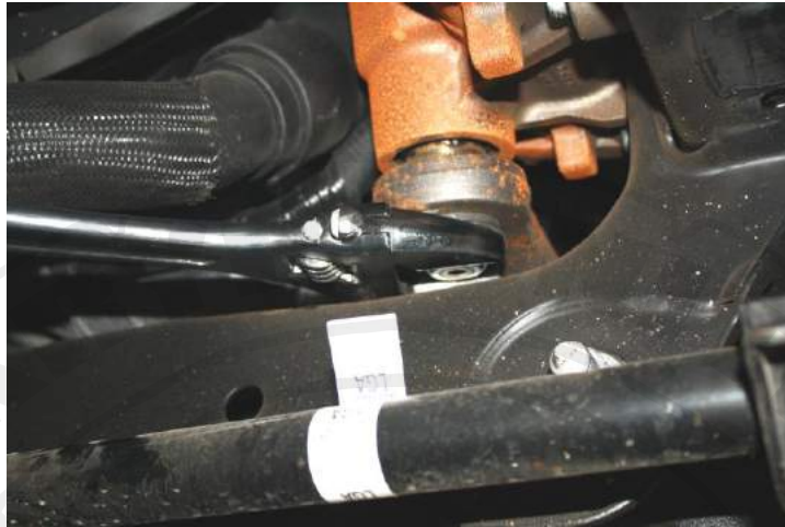
Figure 5: remove large nut and washer holding pitman arm onto steering box
