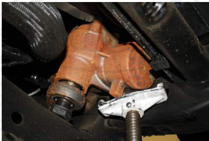
Figure 7: prop the steering box up away from the cross member
