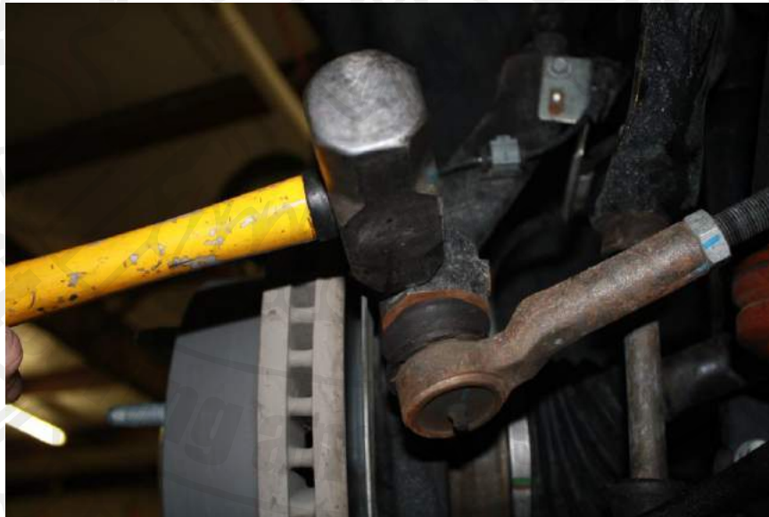
Figure 9: remove passenger tie rod from spindle
