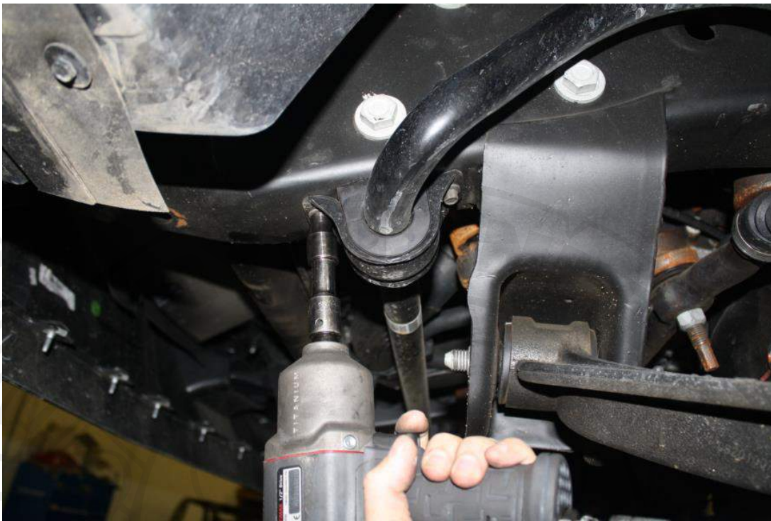
Figure 3: unbolt sway bar from frame
