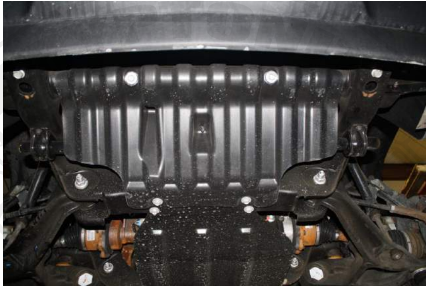
Figure 1: shroud and skid plate
