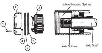
6. Grasp the spirolox (Item 6) and spread it apart with your fingers. Angle the entire lock ring (Item 5) away from face of the body assembly so that the inboard can be inserted into the ring groove in the truck. Maintain the angle and continue to insert the lock ring in a spiral manner until the lock ring is installed. Insert into the groove of the wheel housing. These hold the body assembly into the housing.
