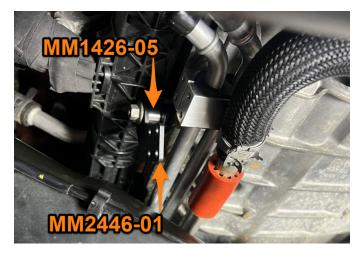
16. Fasten MM2446-01 to MM10014 using the provided M4 bolts.(4x BF4X0.7-10B)
