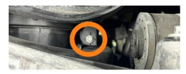
**51.** Unplug the horn wire harness connector, then unclip the wiring harness from the grille support structure.
