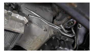
14. Place MM10013 over the two transmission lines at the front of the engine, then clamp MM10014 over the top of MM10013.(1x MM10013, 1x MM10014)
