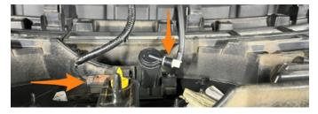
**45.** Remove the 13mm bolt securing the bottom of the headlight to the body of the vehicle. Do this on both sides.
