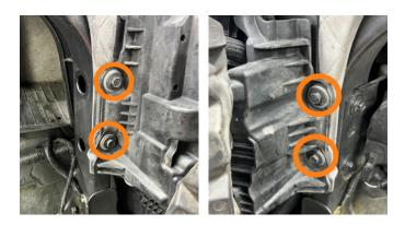
**57.** Remove the tree clips at the top outer corners of the grille support structure's inner ducts. Once the tree clips are removed, remove the grille support structure from the vehicle.
