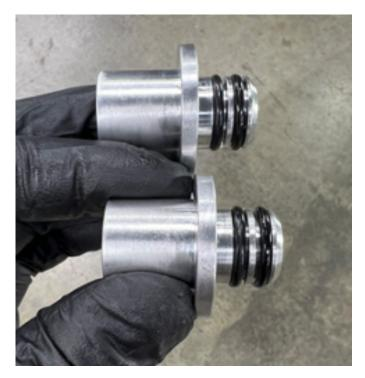
**25.** Install the MM10021-02 fittings into the ports on the side of the transmission. Place MM10021-01 over the fittings and secure them using one of the provided M8 bolts. Use Loctite Blue 242 on the threads of the M8 bolt and torque to 177 lb.in (20Nm). (1x MM10021-01, 2x MM10021-02, and 1x HF8X1.25-25A)
