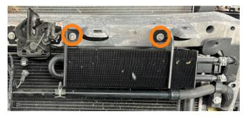
**65.** Place MM1666-01 and MM1666-02 onto each power steering cooler mount, as shown in the image below. Once done, secure the power steering cooler using the previously removed 10mm bolts. (2x MM1666-01 and 2x MM1666-02) (Image on next page)
