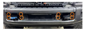
**64.** Remove the 10mm bolts securing the power steering cooler to the radiator support.
