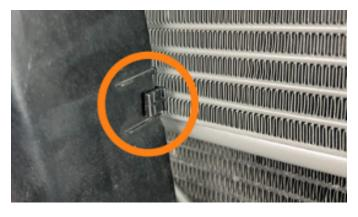
87. Remove the hose routing clip from the front camera washer hose.
