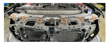
**56.** Remove the 13mm bolts securing the sides of the grille support structure to the radiator support. (Images on top right)
