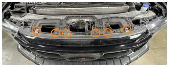
**40.** Remove the lower grille trim cover using a plastic trim panel tool to release the clips securing it in place.
