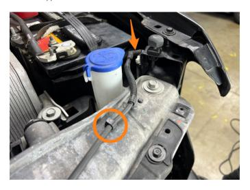
**54.** Remove the tree clips securing the lower radiator ducting to the grille support structure.
