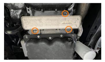
8. Remove the nut securing the front section of the battery wire harness to the passenger side of the engine. (1x 10mm nut)
