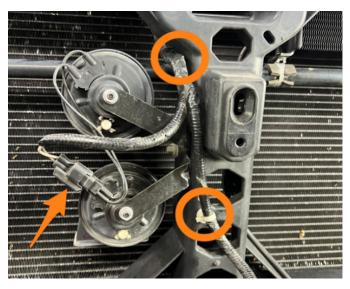
**52.** Unplug the harness connector located under the hood latch assembly.
