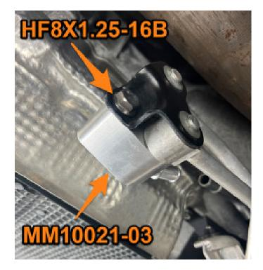
**29.** Reinstall the transmission pan heat shield, then install MM2446-05 to both the transmission and MM10021-03. Torque all fasteners to 80 lb.in (9Nm). (MM2446-05, 3x 10mm nuts, and 2x HF6X1.0-16D)
