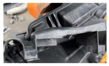
**84.** Mark the area shown in the image below onto the driver-side grille support structure inner duct. Using a razor knife or scissors, cut out the marked area.
