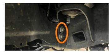
**63.** Remove the 18mm bolts securing the front bumper to the chassis. Once removed, remove the bumper from the vehicle.
