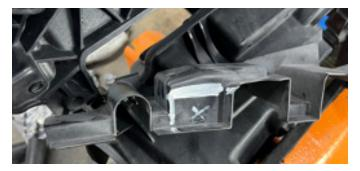
**83.** The image below shows how the passenger-side grille support structure inner duct should look after being modified.
