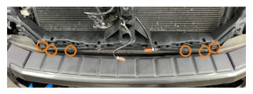
**55.** Remove the 10mm bolts securing the top of the grille support structure to the radiator support.
