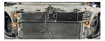
**67.** Loosely install MM1664-02 onto the passenger side of the secondary radiator, as shown in the image below, using two of the provided M6 bolts. Loosely install MM1664-01 onto the driver side of the secondary radiator, as shown in the image below. Fasten MM1660 between MM1664-01 and MM1664-02 using the provided M6 bolts. Tighten all the bolts. (1x MM1660, 1x MM1664-01, 1x MM1664-02, 3x HF6X1.0-20A, and 4x HF6X1.0-14)
