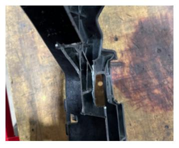
82. Mark the area shown in the image below onto the passenger-side grille support structure inner duct. Using a razor knife or scissors, cut out the marked area.
