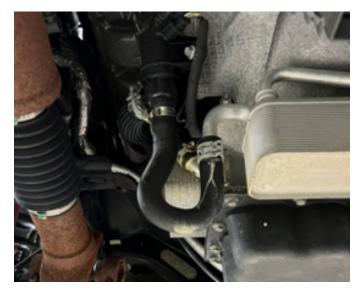
5. Remove the transmission pan heat shield from the passenger side of the transmission by removing the three nuts that are securing it in place. (3x 10mm nuts)
