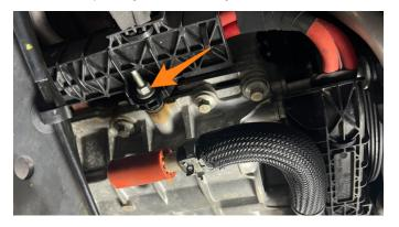
9. Remove the nut securing the coolant line and rear section of the battery wire harness to the passenger side of the engine. Once the nut is removed, remove the coolant line bracket from the stud. (1x 10mm nut)
