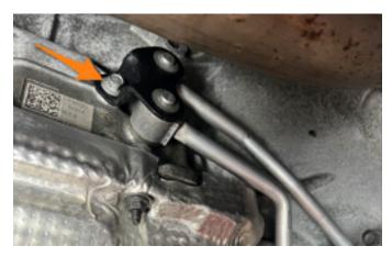
7. Remove the three bolts securing the stock transmission cooler to the bottom of the transmission. Once the bolts are removed, remove the stock transmission cooler from the transmission. Have a drain pan ready to catch any fluid spillage. (3x 13mm bolts)
