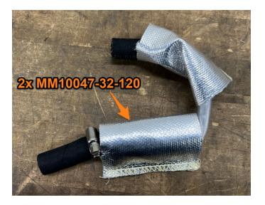
**35.** Connect the line assembly created in steps 33 and 34 to the upper MM10021-02 fitting and upper port on MM10021-03. Secure the line using two of the provided worm gear clamps. Once secured, carefully slide the MM10047-32-120 heat sleeves over the hoses and clamps. (2x MM1325-2)
