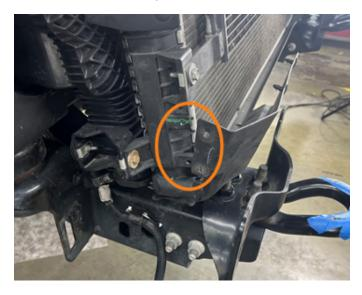
**69.** Route MM4650-02 and MM4650-03 behind the primary radiator, between the fan shroud and the chassis.
