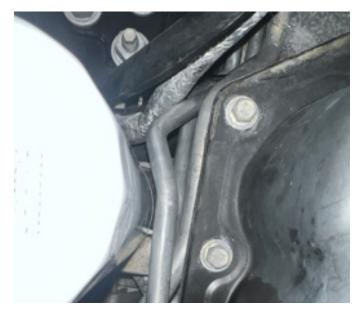
**23.** Confirm that the Mishimoto transmission lines are not contacting the oil pan, coolant line bracket, or other objects along their routing path.
