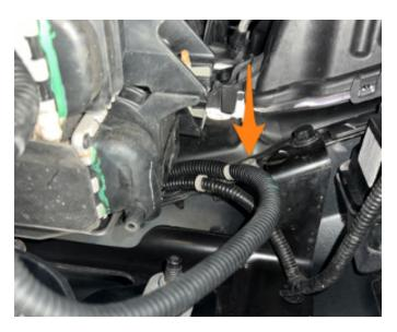
**60.** Unclip the block heater plug from its mount in the front bumper opening.
