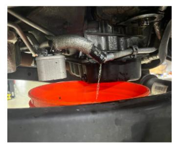
4. Remove the two clamps securing the coolant hose to the driverside coolant line on the stock liquid-to-liquid cooler. Partially remove the coolant hose from the line to allow any residual coolant left in the primary cooling system to drain in a controlled manner. Once drained, remove the hose from the stock liquid-to-liquid transmission cooler.
