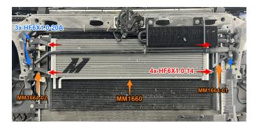
**68.** Remove the tree clips securing the passenger side of the lower radiator duct to the secondary radiator.
