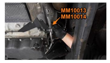
20. Fasten MM2446-02 to MM10014 using the provided M4 bolts.(4x BF4X0.7-10B)
