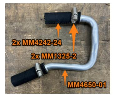
**34.** Slide one MM10047-32-120 over each end of the line assembly created in the previous step. (2x MM10047-32-120) (Image on next page)
