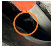
**10.** Feed MM4650-05 behind the coolant line and between the engine oil pan and engine cradle. It is best to feed the transmission line into this area through the gap between the passenger-side radius arm and frame. This line will route transmission fluid along the side of the engine, between the engine oil pan and the coolant line.
