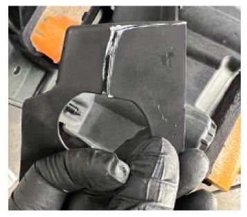
**85.** The image below shows how the driver-side grille support structure inner duct should look after being modified.
