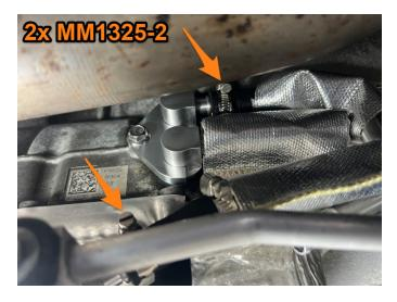
**36.** Slide MM10047-32-170 onto MM4650-05. Install MM4242-67 onto MM4650-05 and the lower port on MM10021-03. Secure the hose using two of the provided worm gear clamps. Once the hose is in place, carefully slide the MM10047-32-170 over top of the hose and hose clamps. (1x MM10047-32-170, 1x MM4242-67, and 2x MM1325-2) (Image on top right)
