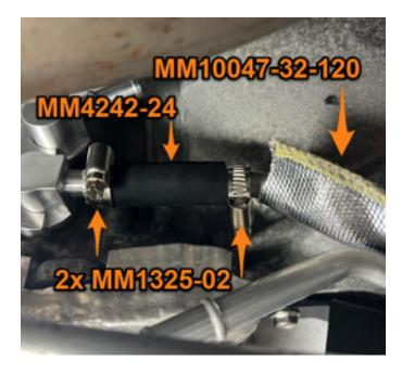
33. Attach one MM4242-24 to each end of MM4650-01 and secure it using two of the provided worm gear clamps.
