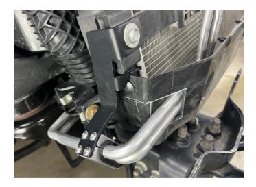
**79.** Mark the area shown in the image below on the passenger side of the grille support structure. Using an angle grinder, cut out the marked area.
