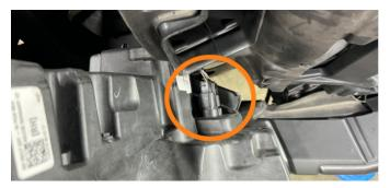
**48.** Remove the two tree clips securing the lower air intake duct to the grille support structure.
