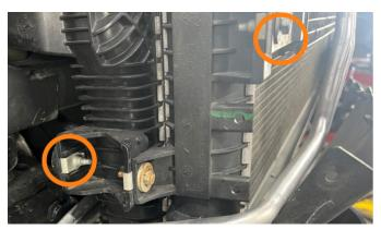
**72.** Install MM2446-03 onto the lower AC condenser mount using the previously removed bolt.
