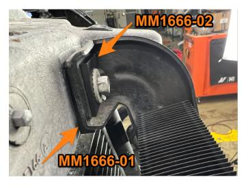
**66.** Remove the 10mm bolt from the upper passenger-side AC condenser mount and the two 10mm bolts securing the coolant line that crosses in front of the secondary radiator.
