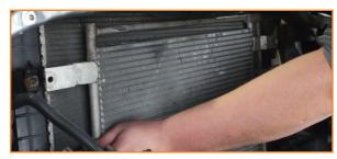
Install the stainless steel hose barbs provided in your kit to the transmission cooler hoses.
