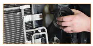
7. Mark the transmission cooler hoses. It's recommended that the mark be five inches back from the hump. Once done, cut the hoses on your mark.
