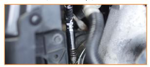
4. Remove the bolts on the upper brackets that secure the intercooler. (2x 10mm bolts)
