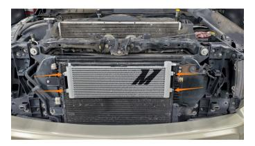
**9.** If the Mishimoto transmission cooler is being installed in addition to the stock transmission cooler, transfer one of the dust caps from the stock transmission line onto the longer of the two supplied transmission lines. Then, install the longer of the two supplied transmission lines to the driver-side port on the Mishimoto cooler and, using a flathead screwdriver, secure it with one (1) of the supplied worm gear clamps. [Image on top right]
