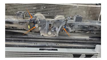
**12.** Drill a ¾" hole through the shroud on the mark that was made in Step 10. Then, reinstall the shroud and hood latch. Check that the hood closes and latches properly. Adjust the position of the hood latch if necessary.
