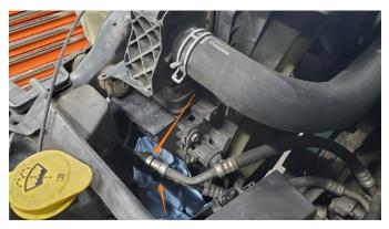
6. Using a 10mm socket remove the three (3) bolts securing the stock transmission cooler to the intercooler.
