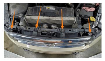
3. Remove the hood release cable from the plastic clip, remove the two (2) trim clips securing the plastic shroud to the frame, and slide the shroud out of the way.
