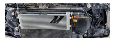
**18.** Transfer one (1) dust cap from the stock transmission lines to each of the Mishimoto lines and connect the Mishimoto lines to the vehicle where the stock lines were disconnected and install the dust caps over the connections.
