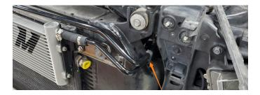
**20.** Using a 13mm socket, remove the upper fan shroud bolt and install the supplied line bracket in this location. Attach the supplied p-clip to the upper factory transmission line and secure it to the line bracket with the supplied M5 bolt and lock nut.
