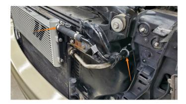
**10.** Position the plastic shroud that was slid out of the way in Step 3 back into place. Then, make a mark on the shroud directly above the fitting on the passenger-side of the stock transmission cooler.
