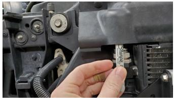
**11.** After making the mark, remove the shroud from the vehicle to be drilled by removing the plug from the hood latch. Then, using a 10mm socket, remove the two (2) bolts securing the hood latch to the frame so the shroud can be slid off the hood release cable. Marking the position of the latch on the frame before removing it will help to reinstall it in the correct position. (Image on next page)
