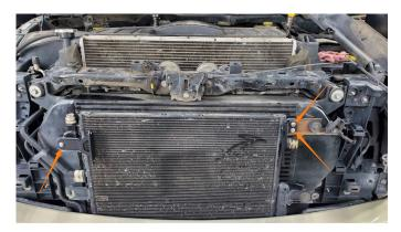
8. Attach the Mishimoto transmission cooler to the mounting brackets with the four (4) supplied 10mm long M6 hex head flanged bolts. Then tighten the bolts securing the mounting brackets to the vehicle. If the Mishimoto transmission cooler is being installed to replace the stock cooler (with the optional bypass line kit, sold separately), skip to Step 15.
