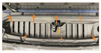
3. Remove the 1X push clip and 1X harness clip for the intake duct.
