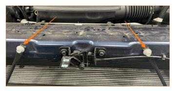
5. Remove the plastic cap that covers the fitting on the inlet and outlet of the transmission cooler by pushing it away from the cooler. Then, use a pick tool or similar to remove the metal clip that secures the line into the transmission cooler fittings (Shown outside of the vehicle).
