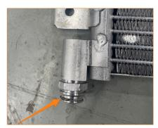
6. Place towels or other oil-absorbent material underneath the transmission cooler fittings. Then, remove the 1x 10mm bolt securing the transmission cooler to the cooling stack on the passenger side. Finally, work the transmission lines free from the transmission
