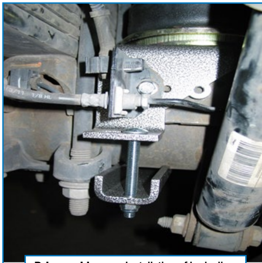
Drivers side rear. Installation of brake line.
