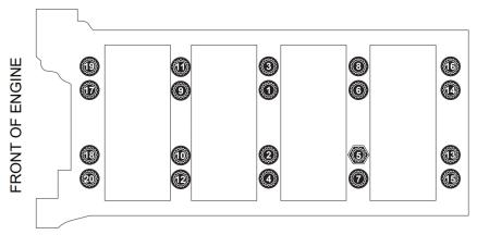
Install the Oil Pickup Tube, make sure the mount is installed over the stud on Position #5. Lubricate the M10 Nuts with the Assembly Lubricant provided. Install the M10 Nut and M10 Washer onto the stud in Position #5.
