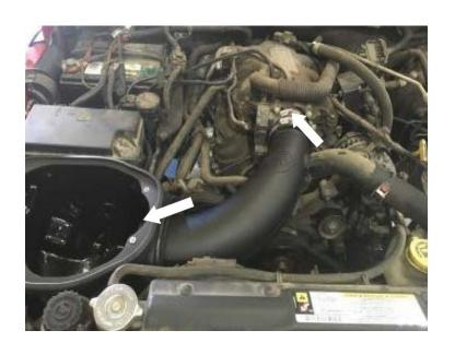
Install the Air Filter (F) into the Intake Tube (J) and tighten Hose Clamp #72 (G).
