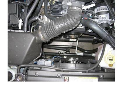
Lift up to unseat the prongs from the grommets on the airbox tray and remove the stock intake assembly from the vehicle.
