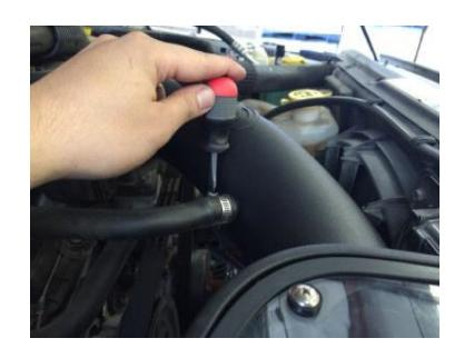
Reconnect the IAT sensor harness into the IAT sensor and engage the red locking clip.
