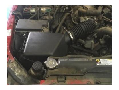
Install the Tube Seal (I) onto the Airbox (H).
