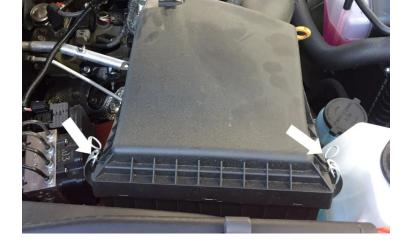
Remove the three screws securing the stock airbox with a 12mm Socket/Wrench. These screws will be reused in Step 16.
