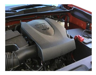
Unfasten the MAF harness wire from the clip on the airbox lid and pop out the clip on the resonator.
