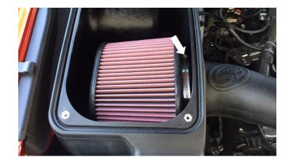
Press the Lid Seal (G) into the grooves on top of the Airbox (A).
