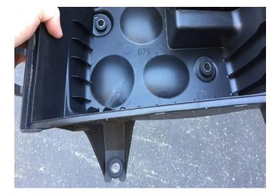
Install the grommet into Airbox (A) first and then the metal bushing.
