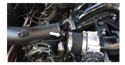
Reconnect the CCV hose and hose clamp into the CCV vent on the Intake Tube (B).
