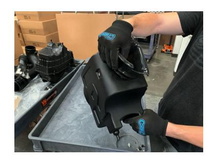
Install the Lid Seal (F) into the groove on top of the Intake Box (A). Cut away any excess lid seal.
