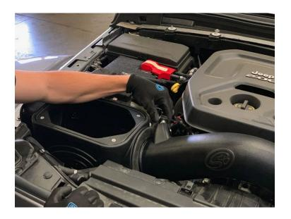
Install the Air Filter (E) and #80 Hose Clamp (M) onto the Intake Tube (B) then tighten the hose clamp. Do not overtighten.
