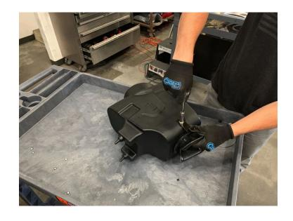
Install the Intake Box (A) into the vehicle, making sure the prongs align with the two grommets, then push down on the intake box to fully seat the prongs.
