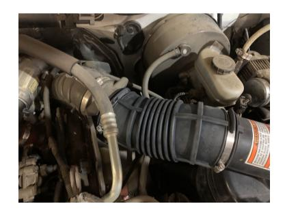
Remove the 2 fasteners on the stock airbox lid.
