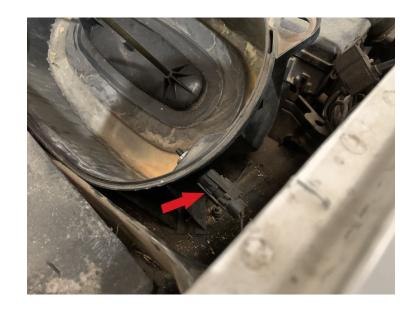
Pull up to remove the stock airbox.
