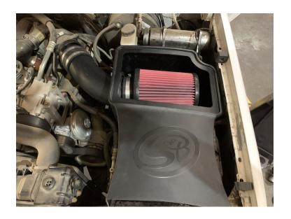
Slide the Coupler (E) onto the baffle and tighten both Hose Clamps (J).
