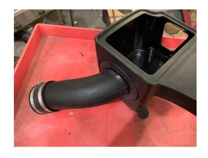
Install the Air Filter (C) loosely onto the Intake Tube (D).
