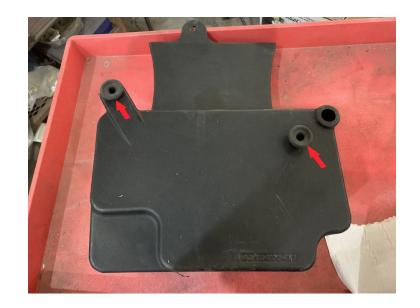
Install the Tube Seal (B) onto the Airbox (A).
