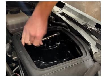
Install the fuse box onto the bracket if your truck is equipped with one.
