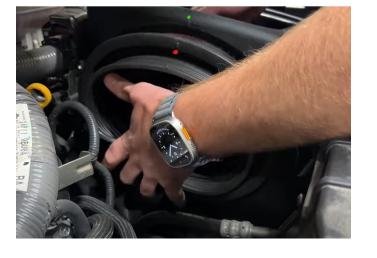
Install the front silicone scoop into the S&B airbox with the airbox in the truck
