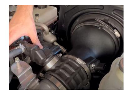
Reinstall the MAF connector to the sensor.
