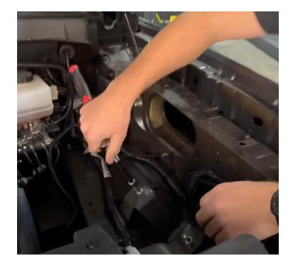
Install the IAT sensor grommet onto the S&B tube, make sure the tab lines up with the notch on the tube.
