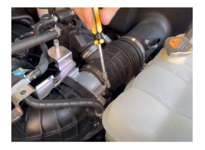
Remove the hose clamp holding the baffle to the intake tube and separate it from the tube
