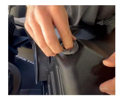
Remove the MAF sensor from the OEM intake tube. Place the MAF sensor through S&B MAF gasket & plastic pad. Use the included S&B bolts to secure the sensor to the S&B intake tube.
