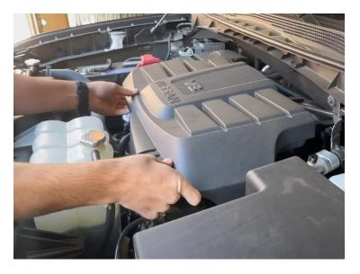
Depress the button on the MAF sensor connector and remove from the MAF.
