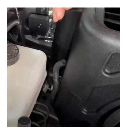
Remove the S&B lid from the protective film and install it into the S&B lid trim. Press the S&B snap in lid into the airbox.
