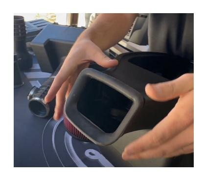
Remove the metal bushing and gromet from the OEM airbox and install it onto the S&B airbox next to the side inlet.
