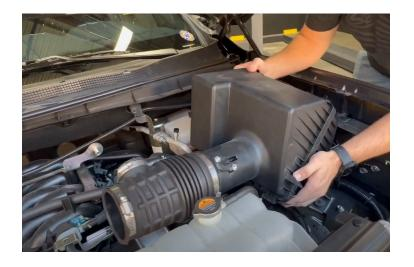
With a panel popper, remove the pins holding the side inlet to the body.
