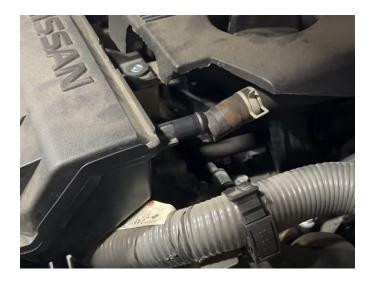
Depress button on the MAF sensor and remove.
