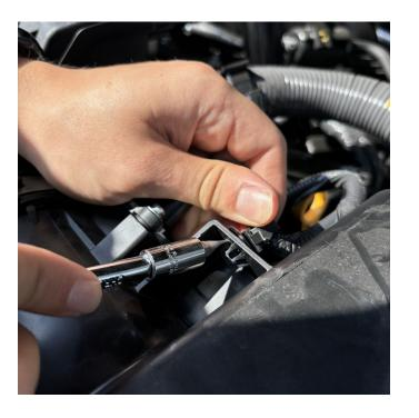
Remove the intake tube/box from the vehicle.
