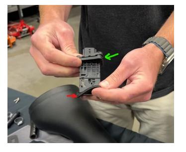
Remove the 2 large grommets from the OEM intake and install onto the S&B airbox.
