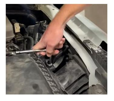
Loosen the hose clamp on the throttle body.
