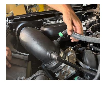
Attach the Air Box Inlet to the Air Box.
