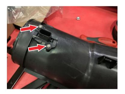
Using the MAF gasket and MAF plastic pad install into the S&B intake tube with the included longer Phillips head bolts.
