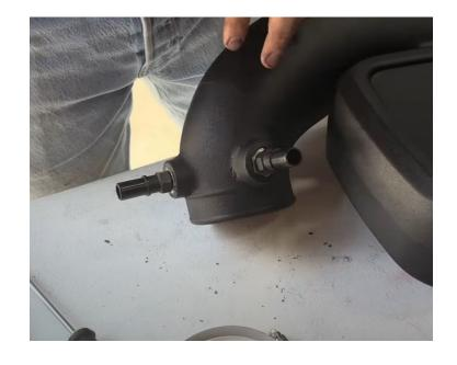
Tighten the quick-connect fittings onto the tube using a wrench. Do not over-tighten. It is normal for threads to still be showing on the fittings.
