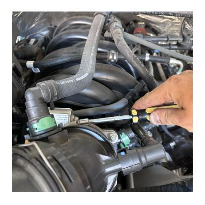
Disconnect the vent lines from the stock intake tube. Please watch our install video if you have questions on how to remove the quick connects.
