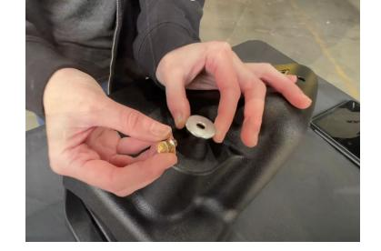
With a 10mm socket install the bracket onto the front of the airbox
