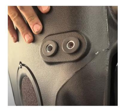
Install the S&B tube seal into the S&B airbox
