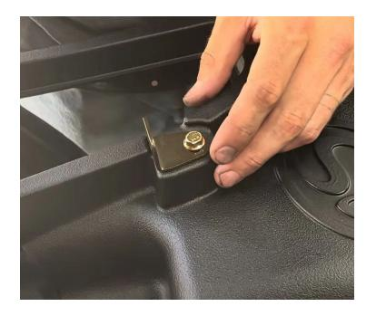
Install foam inserts into the airbox. The plastic plate will hold the foam in place.
