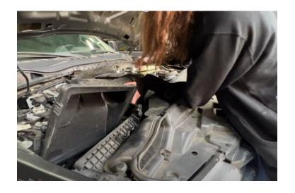
Carefully remove the stock intake filter.
