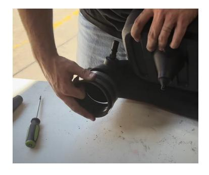
Install the intake tube through the airbox and rotate the tube down until the coupler is on the throttle body and the resonator mounting stud is seated.
