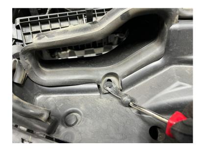
With a 8mm socket and extension, remove the bolt holding the front of the intake to the vehicle. Then remove the intake box from the truck.
