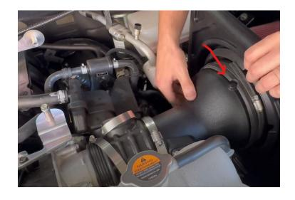
Install the baffle into the S&B coupler and tighten down all the hose clamps
