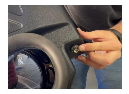
Install the S&B airbox into the truck
