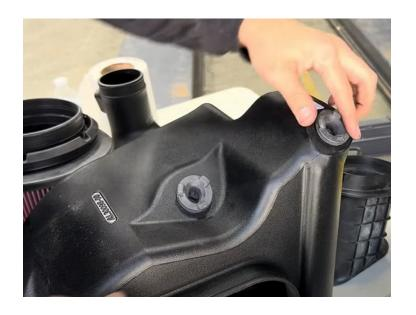
Install the S&B silicone side scoop onto the airbox
