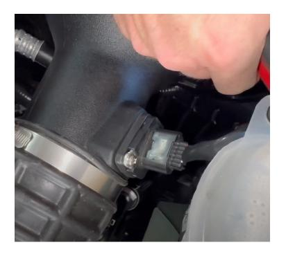
Cut off the OEM Christmas Tree and install the S&B Christmas Tree pin and install into the hole on the S&B airbox.
