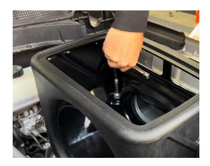
Remove the MAF sensor from the OEM intake tube. Place the MAF sensor through S&B MAF gasket & plastic pad. Use the included S&B bolts to secure the sensor to the S&B intake tube.
