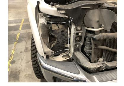
Unclip the headlight harness from the plastic intake scoop and pull the intake scoop up and out of the vehicle.
