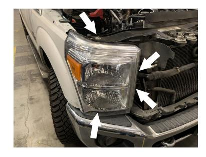
Tools Required: Socket Wrench, 10mm Socket
