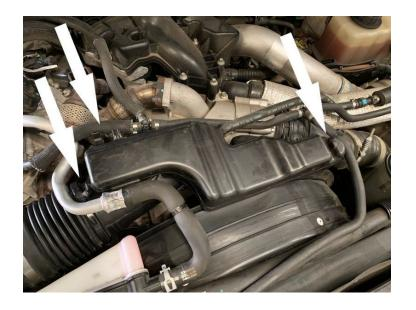
Lift the stock air box up to unseat the grommets from the air box tray and remove the stock air box from the vehicle.
