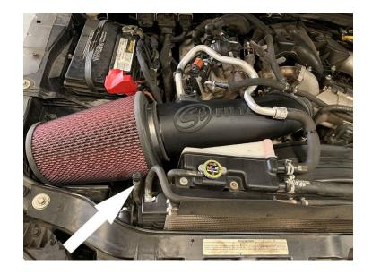
Finish securing the kit to the vehicle by tightening the #74 hose clamp over the coupler and around the turbo inlet.
