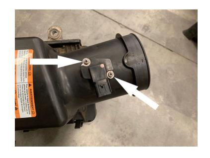
Install the MAF sensor, MAF sensor pad (I) and MAF sensor pad gasket (J) onto the intake tube, securing them to the tube with the provided phillips head screws (H).
