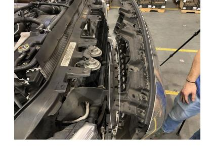
Remove the four screws securing the passenger side headlight assembly to the vehicle and firmly pull the light straight out, unclipping it from the frame of the truck.
