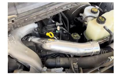
Then connect the intercooler to the boot using a flathead screwdriver and clip the assembly into the turbo. Make sure you hear a click sound when it connects.
