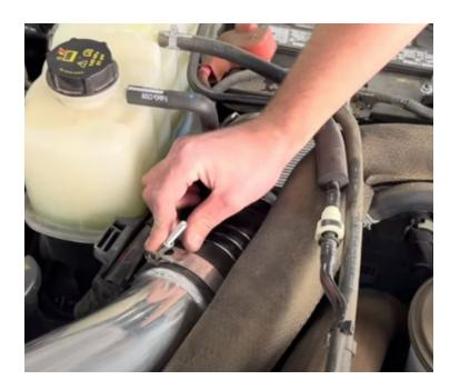
Once the hose clamp springs are installed on the boot, reinstall the springs and nuts then tighten down to 76 Inch-Pounds.
