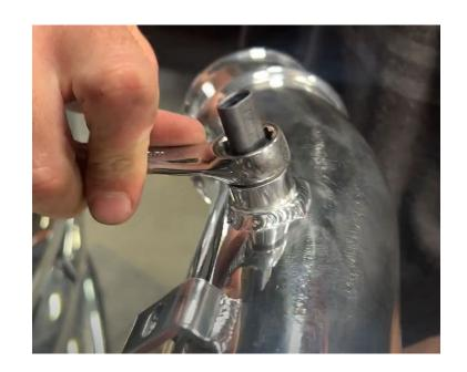
Slightly slide the S&B intercooler onto the collar at the turbo.
