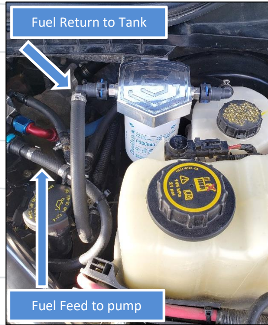
Figure 7: Left Side hose installation (2017+)
