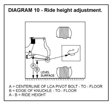
NOTE: When adjusting the torsion bars, always bounce the vehicle after 1-2 rotations of the adjuster bolt. This will reset the torsion bars to the new ride height and will allow more accurate adjustments. Always bounce the vehicle before taking a measurement.
