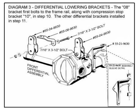
□ Loosely attach the remaining two "04" brackets to the frame. Use the factory bolts, pointing forward. Hand tighten only.
