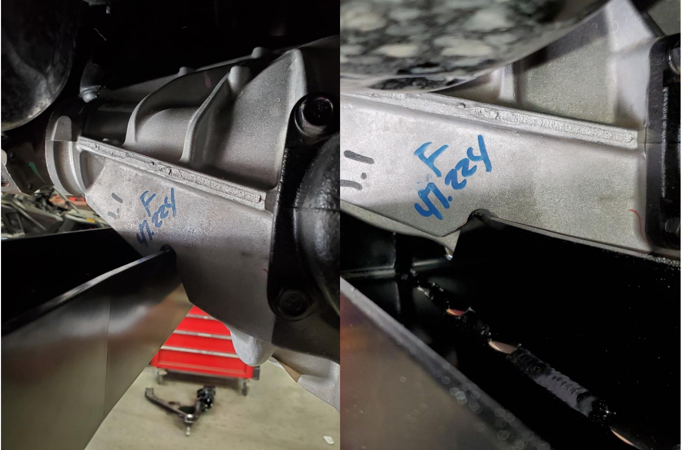
Figure 44: Clearance of rear crossmember.
