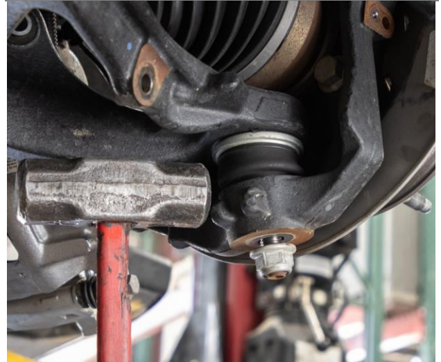
Figure 10: Loosen Lower Ball Joint
