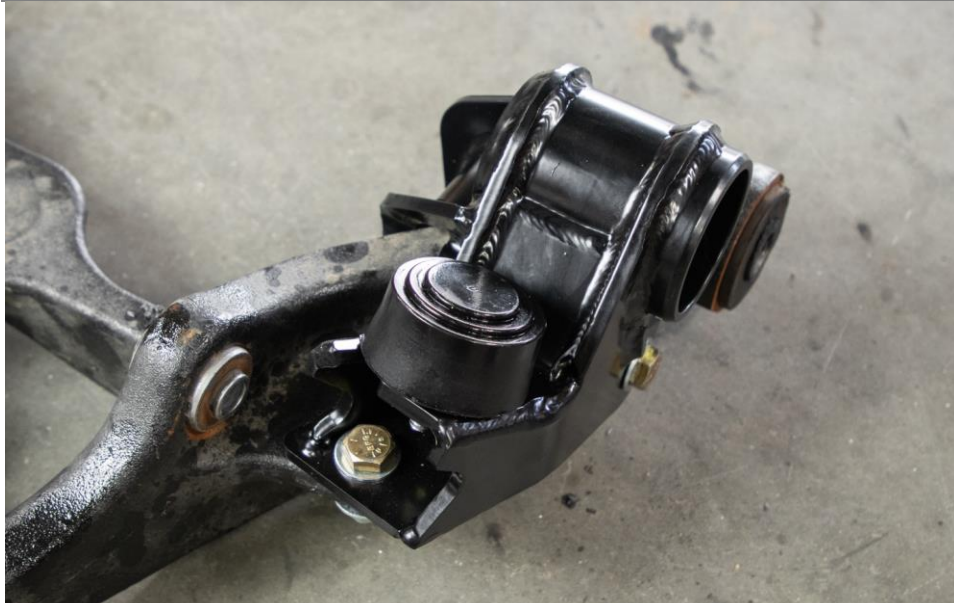
Figure 51: Install Outer Mounting Bolt and Bump Stop
