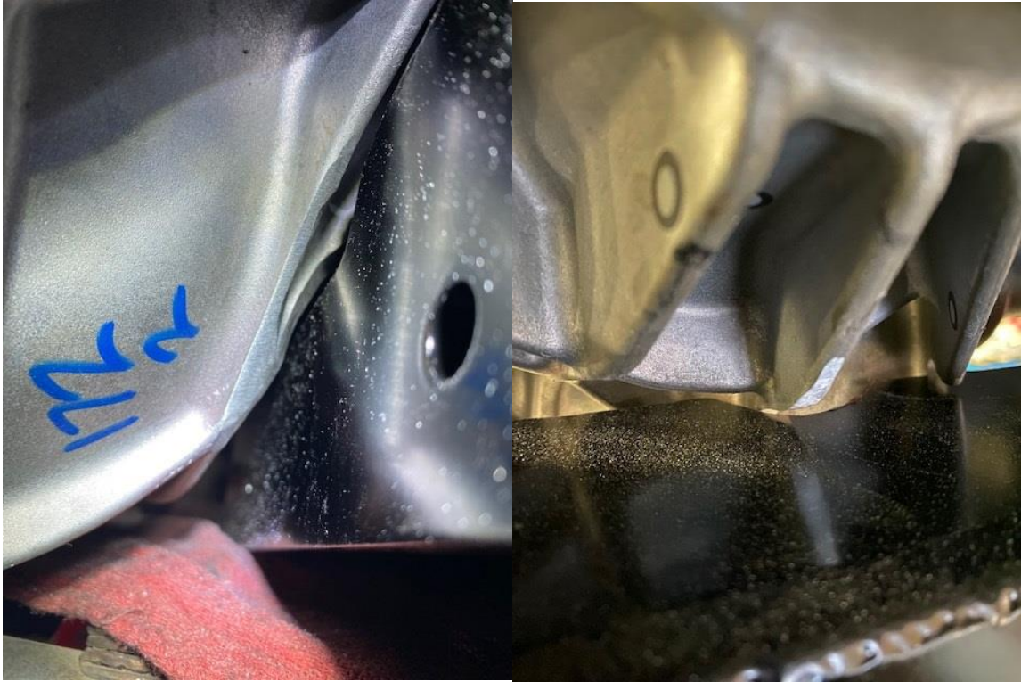
Figure 37: Additional differential housing trimming.
