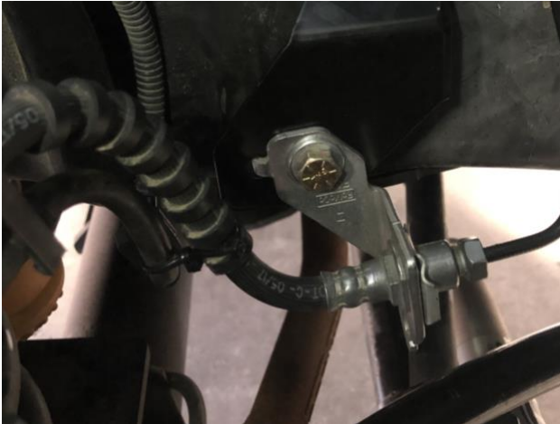
Figure 6: Diver Side ABS Line Installed
