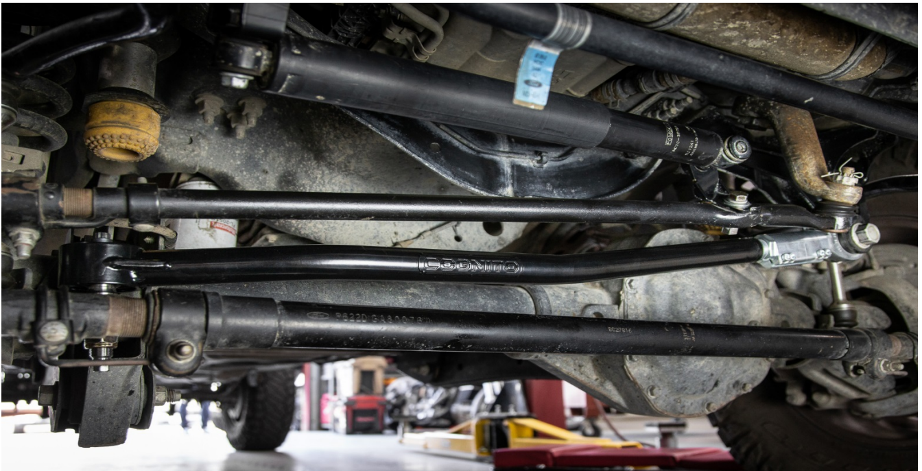
Figure 21: Installed Track Bar
