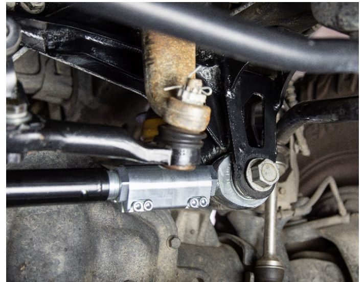
Figure 13: Installed Track Bar
