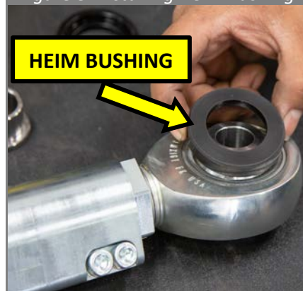
Figure 8: Installing Heim Bushing
