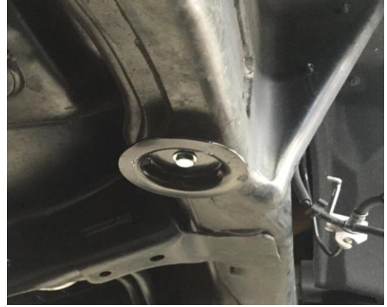
Figure 10B: FSD Bump Stop Spacer Hardware
