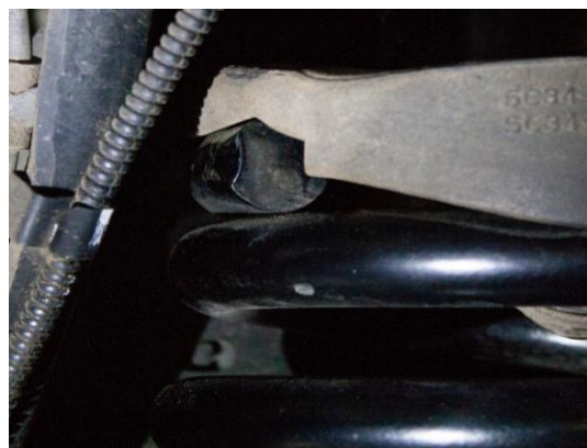
Figure 14A: Coil Spring and Isolator Orientation
