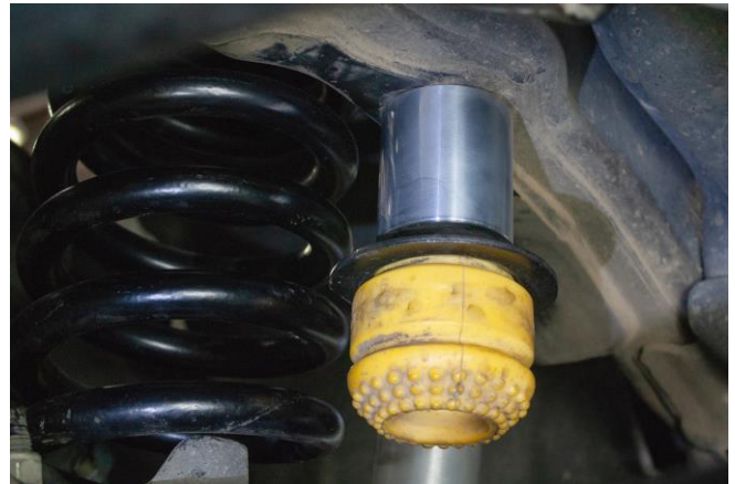
Figure 13: Bump Stop Spacer Orientation
