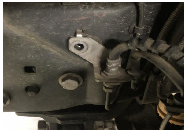
Figure 1B: OE Brake Line Bracket, Bolt Removed
