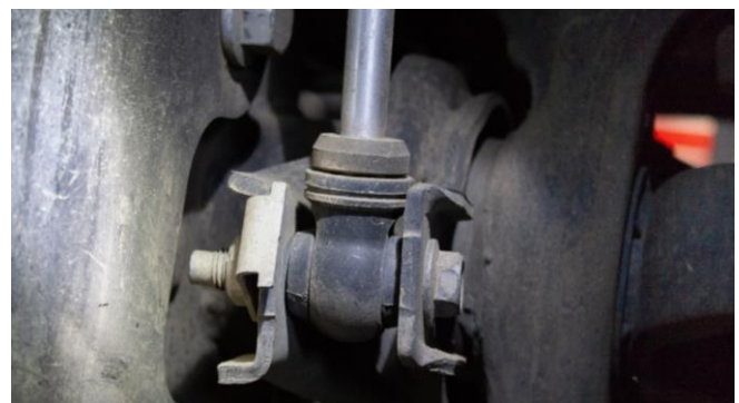
Figure 16B: Front Lower Shock Mount Installed
