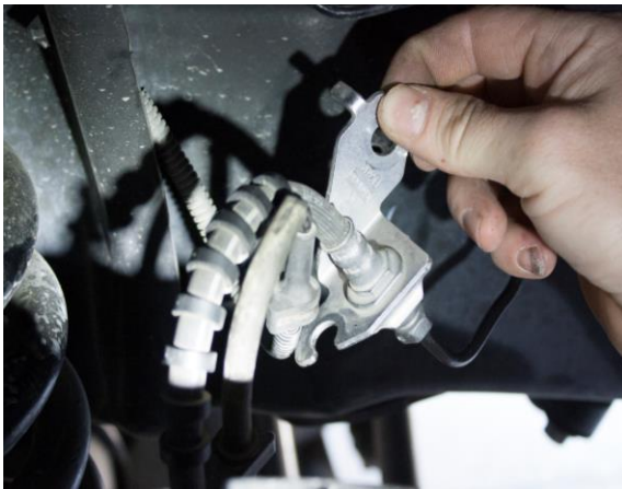
Figure 2A: Passenger ABS Line Removal
