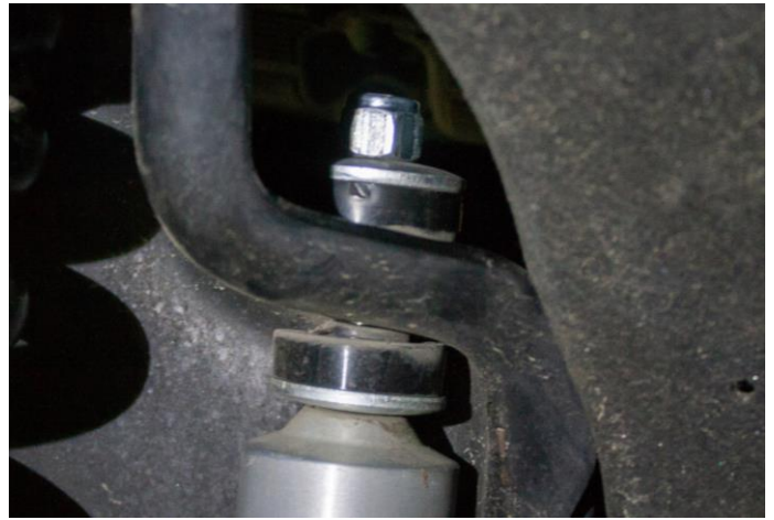
Figure 15B: Top Shock Mount Installed
