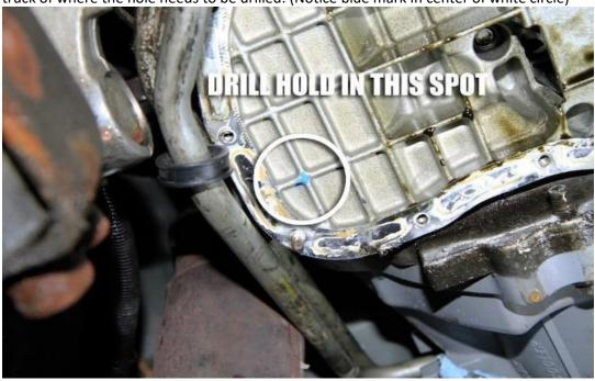
15. Drill a small pilot hole first for the large drill to follow. Then drill with a 37/64" Bit.
